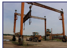
MI JACK (40 & 50) TON TRAVEL LIFT
